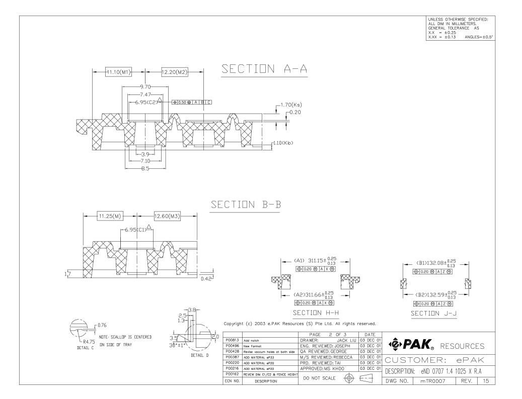
UNLESS OTHERWISE SPECIFIED: ALL DIM IN MILLIMETERS. GENERAL TOLERANCE AS X.X =  $\pm 0.25$ X.XX =  $\pm 0.13$  ANGLES= $\pm 0.5^{\circ}$
