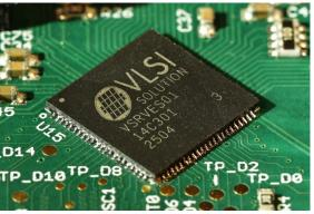
capable of running stock Linux. Linux boot time, including Ethernet networking, is only 2.6 seconds. As a speciality, Linux can be rebooted without interruption of audio playback.
