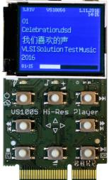
After decoding, audio can be forwarded either digitally to an external decoder, or to the integrated DAC of VS1005.
