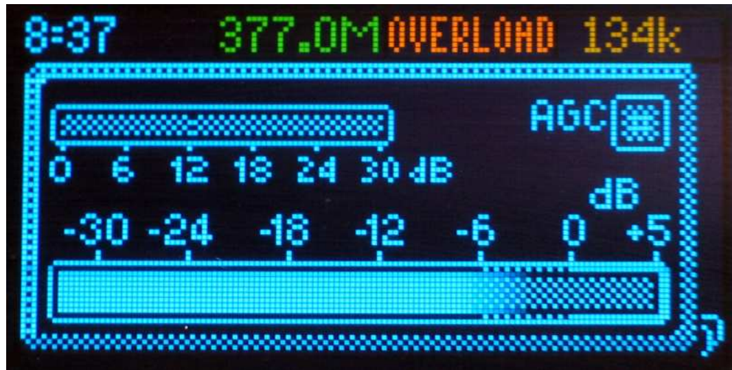
Figure 2.3: Real Record Display with Monochrome VU Meter.
