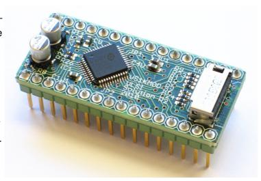
The VS1000 Module is an ideal choice for upgrading a system to be more user friendly. The module can play spoken instructions, music, user manuals etc in multiple languages. Such applications are for instance lifts, ticket machines, vending machines, and car accessories. Alternatively, the VS1000 Module can be used as a standalone player that is triggered by IO pins, UART or USB. These kind of applications are for instance alarm systems, PC accessories and Hi-Tech toys.
