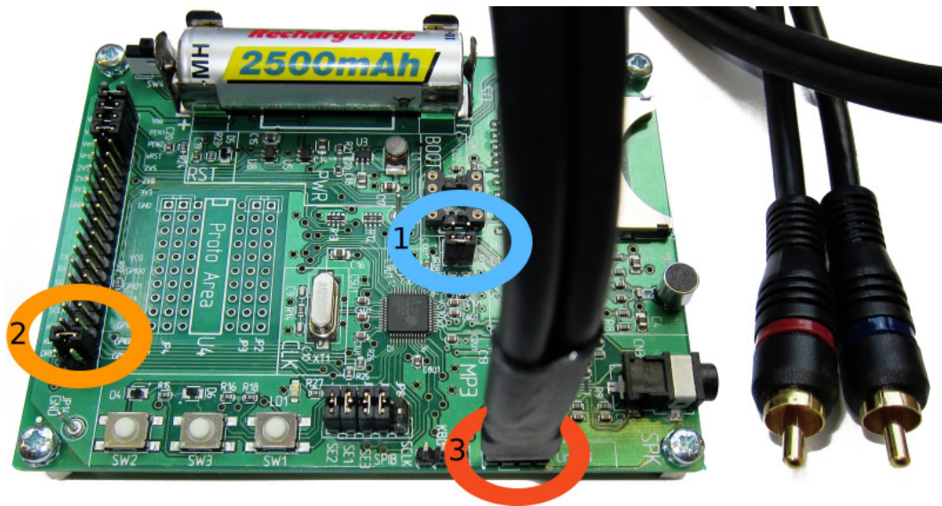
Figure 5: Standalone Recorder configured for stereo line input (cable not included)
