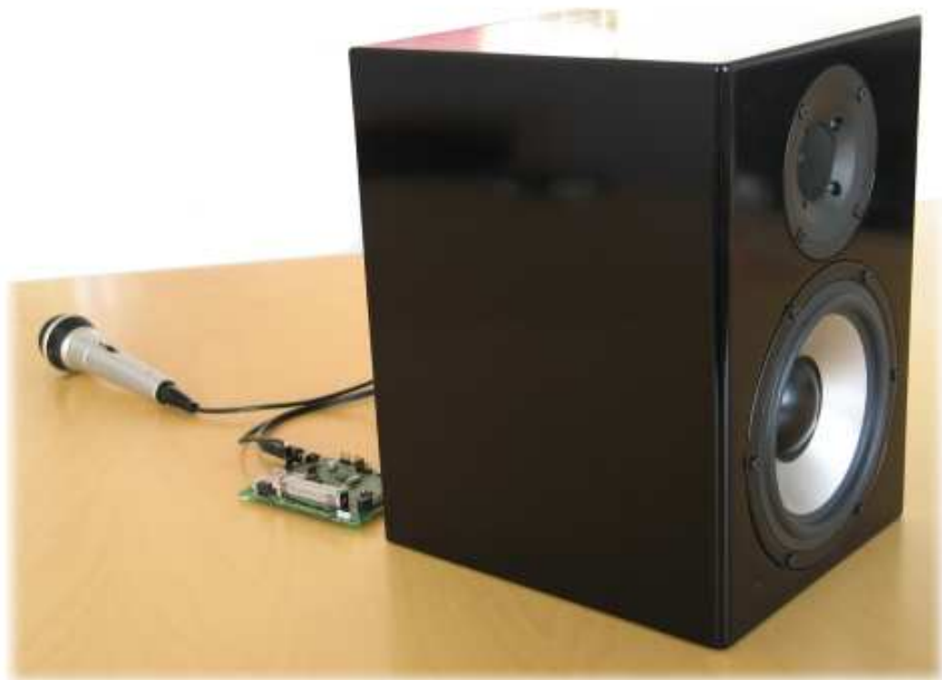
Figure 3.1: VS1103b Feedback Eliminator with Microphone and Active Loudspeaker
