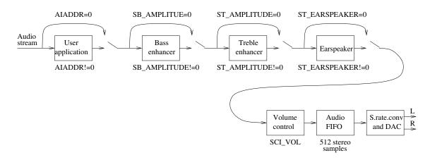
Figure 13: Normal Data Flow of VS1103b, Part 2.
