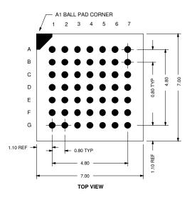
Figure 2: Pin Configuration, BGA-49.
