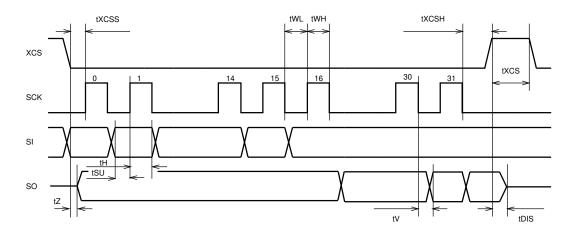
Figure 8: SPI Timing Diagram.
