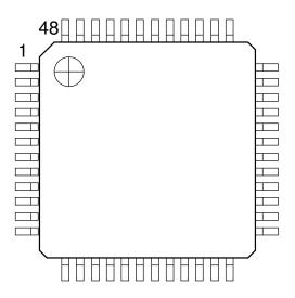
Figure 1: Pin Configuration, LQFP-48.
