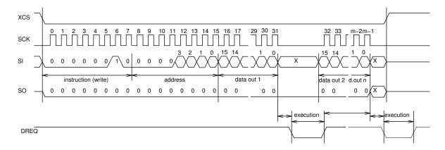
Figure 7: SCI Multiple Word Write
