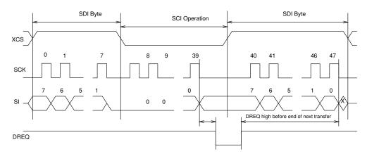
Figure 12: Two SDI Bytes Separated By an SCI Operation.
