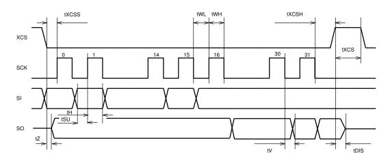
Figure 9: SPI Timing Diagram.
