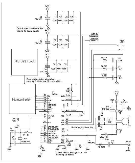
Figure 3: Typical Connection Diagram Using LQFP-48.
