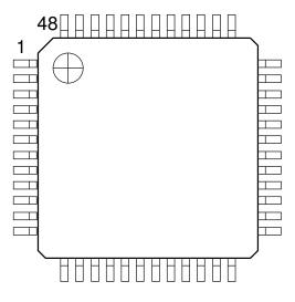
Figure 1: Pin Configuration, LQFP-48.
