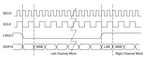
Figure 18: I2S Interface, 192 kHz.
