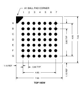
Figure 2: Pin Configuration, BGA-49.
