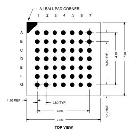
Figure 2: Pin Configuration, BGA-49.
