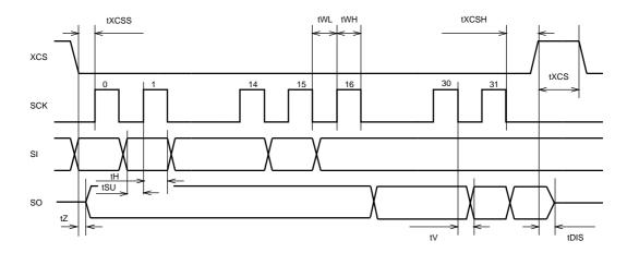
Figure 9: SPI Timing Diagram.
