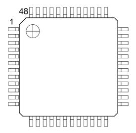
Figure 1: Pin Configuration, LQFP-48.
