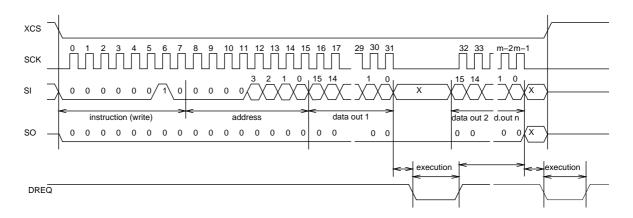
Figure 8: SCI Multiple Word Write
