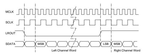
Figure 18: I2S Interface, 192 kHz.
