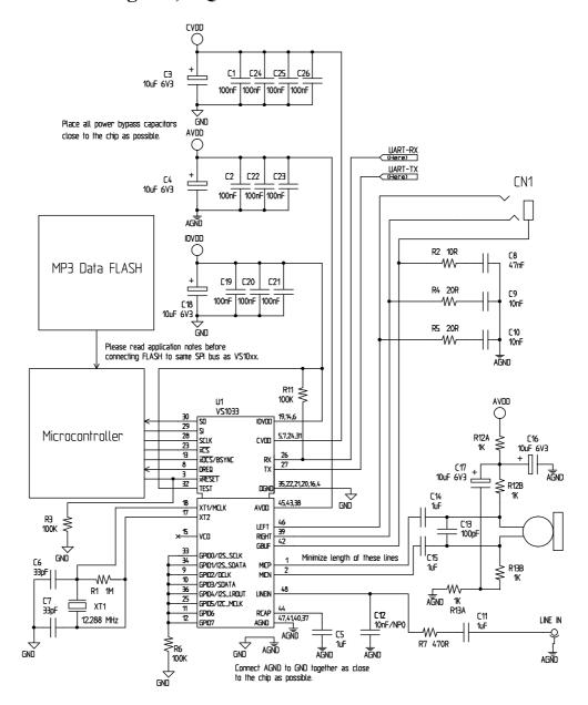
Figure 3: Typical Connection Diagram Using LQFP-48.
