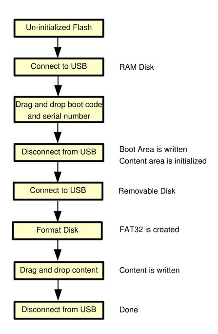
Figure 1: Flash programming procedure for R/W applications
